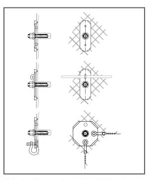
\* Anchor plates with two rope guidances, i.e. in vertical and horizontal directions are also available
