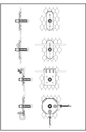
\* Anchor plates with two rope connections, i.e. in vertical and horizontal
