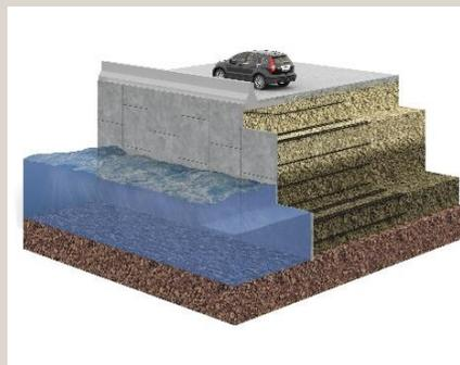
Above: 3D drawing of a Reinforced Earth® structure.
