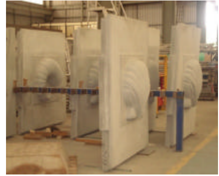
Left: Placing of TerraSet® Shell Pattern panel. Note checking of levels, and clamps ensuring correct panel alignment during construction.
